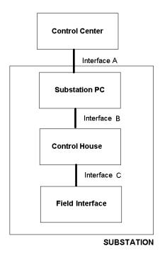
Figure 3 IED Layers and interfaces of communication infrastructure in the substation
