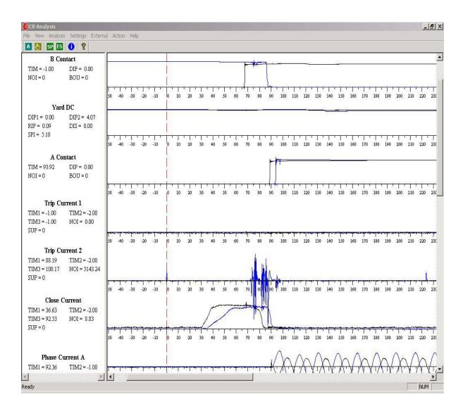
Figure 10 CBM signal waveforms displayed using CBMA Viewing software
