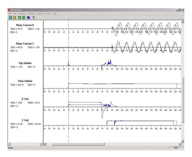
Figure 11 CBM signal waveforms displayed using CBMA Viewing software (continued)
