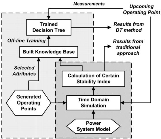
Fig. 3. Comparison between conventional approach and the DT method
