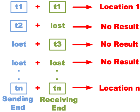
Figure 2. Impact of packet loss on two-terminal fault location algorithm
