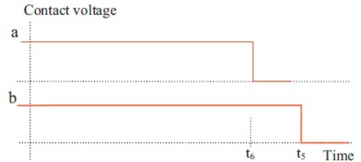
Fig. 3. 'a' and 'b' contacts transition during opening
