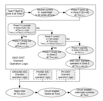
Fig. 2. Reasoning process for building relay operation logic
