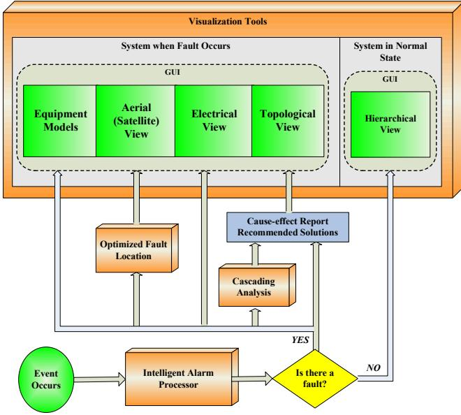
Fig. 4: Functions of Visualization Tools
