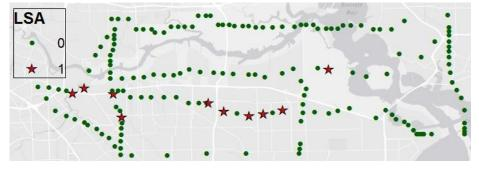
Fig. 5. Optimal locations of line surge arresters base on risk analysis.
