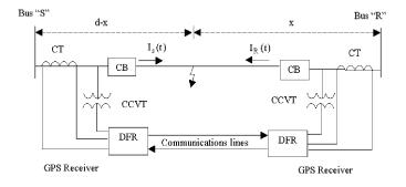
Fig. 8. Two ended fault location setup
