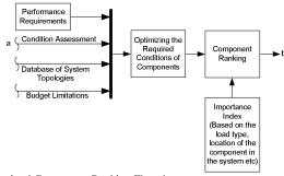
Fig 6: Optimal Component Ranking Flowchart
