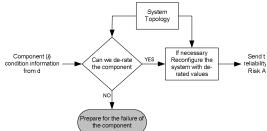
Fig.9: Component Derating and Reconfiguration
