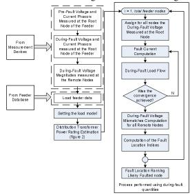
Fig.10 Flow chart of voltage-sag based algorithm [16]
