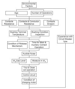
Fig. 4: Topology of SF6 Circuit Breaker
