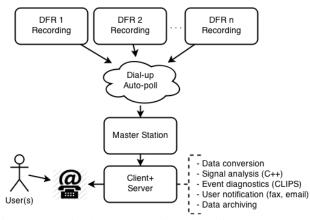
Fig. 4. Centralized system solution using dial-up (~30 DFRs)
