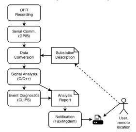
Fig. 2. Single substation field implementation (1 DFR)
