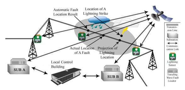
Figure 4: Spatio-temporal correlation of traveling wave fault locator data with lightning, GIS and GPS data
