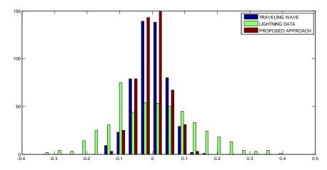
Figure 5: Histogram of an error distribution for individual traveling wave and lightning data; and our approach that combines two methods
