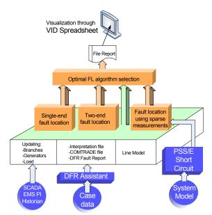
Fig. 8 Architecture of proposed solution
