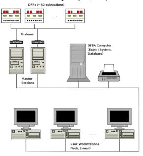
Fig. 1 DFR system for automated fault analysis
