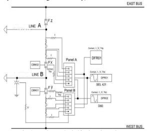
Fig. 3 Breaker and a half substation scheme
