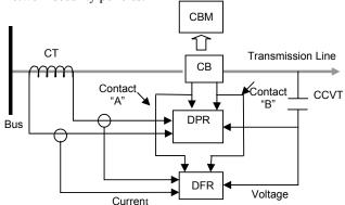
Fig. 4 Example IED configuration on a single line
