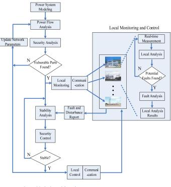
System Monitoring and Control Fig.2 Block diagram of the implementation
