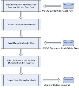
Fig.5 Framework of System Dynamic Stability Analysis
