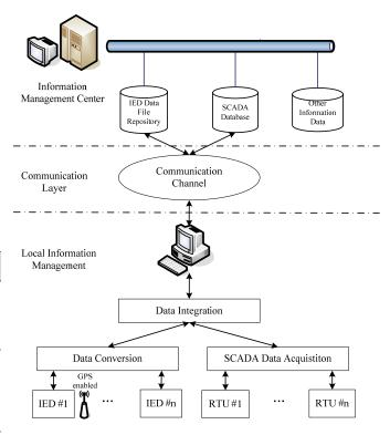
Fig.3 Framework of information management system based on SCADA system and IEDs
