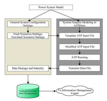
Fig.6 Block Diagram of simulation fault and non-fault scenarios generation
