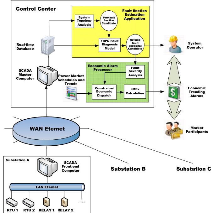
Fig. 8. Intelligent Economic Alarm Processor Architecture
