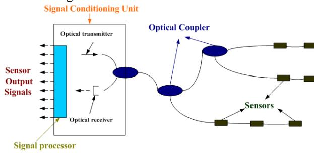
Fig.2. Multiplexing arrangement for FFPI sensors
