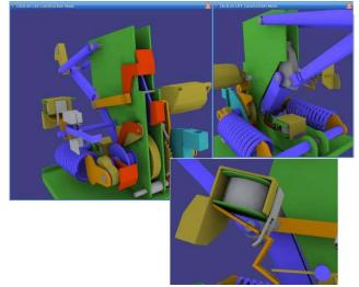
Figure 8: Constructional view of circuit breaker
