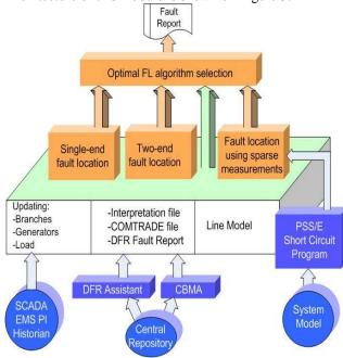
Figure 3: Architecture of fault location module
