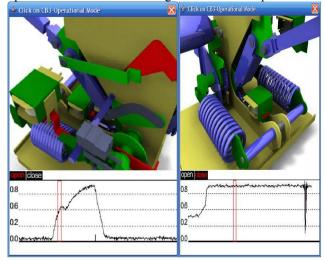
Figure 9: Operational view of opening and closing action of a circuit breaker
