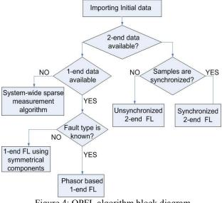
Figure 4: OPFL algorithm block diagram
