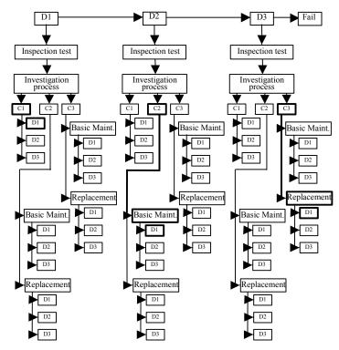
Fig 1. Proposed circuit breaker probabilistic maintenance model.
