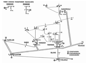
Fig. 3. IEEE-30 bus system diagram.
