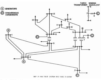
Fig. 2. IEEE-14 bus system diagram.
