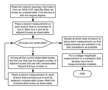
Fig. 1. Flowchart of the branch power flow and voltage magnitude measurement placement.
