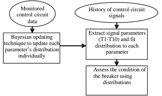
Fig. 3. Failure rate estimation model of circuit breaker
