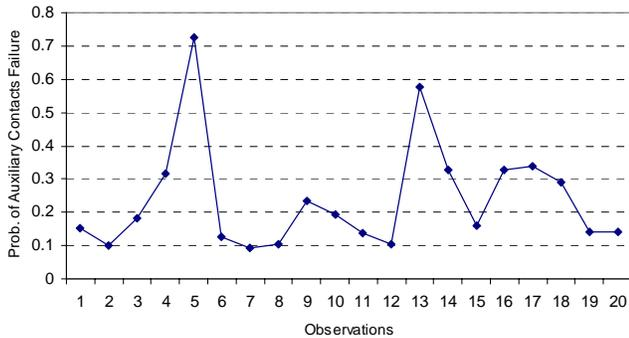
Fig. 11. Probability that the auxiliary contacts fail to operate normally
