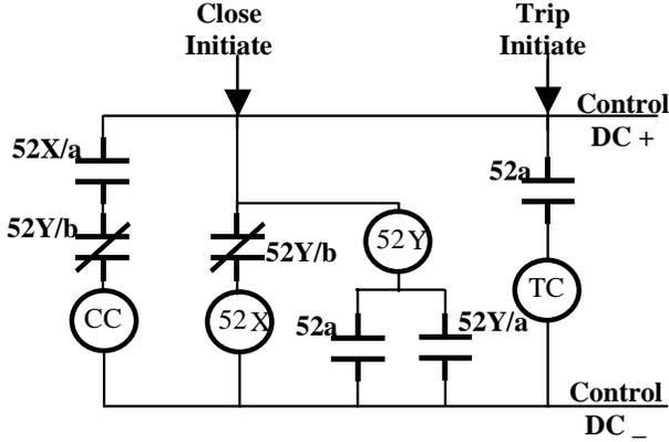
Fig. 1. Electrical representation of circuit breaker control circuit [8]
