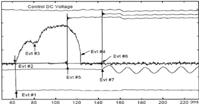
Fig. 2. Control circuit signal during close operation of circuit breaker [22]
