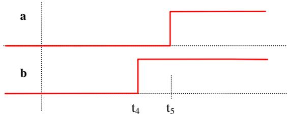
Fig. 10. "a" and "b" contacts transition during close operation
