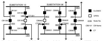
Fig. 5. Diagrams of Substation 6 and Substation 13 in the IEEE 14-bus system.
