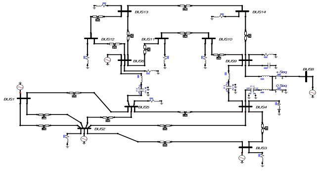
Fig. 2. The IEEE 14-bus system model in ATPDraw.
