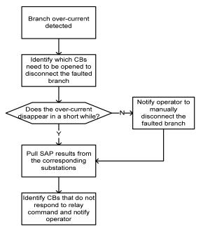
Fig. 4. Analysis procedure of the over-current alarms.
