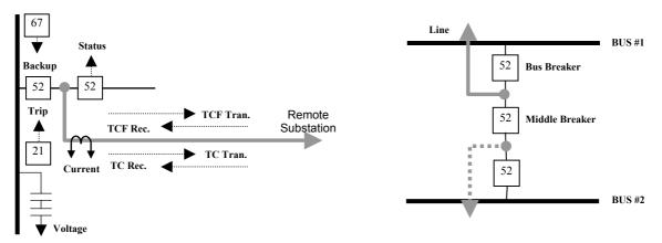
Fig. 1. An example of one line-diagram and the bus-breaker arrangement
