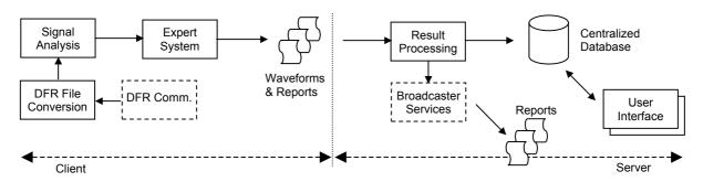
Fig. 2. Client/server architecture of the software for automated analysis
