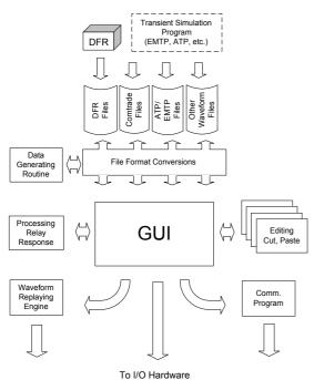
Fig. II. An advanced software configuration for an open-loop simulator
