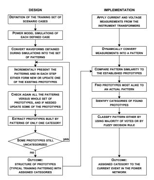
Fig. IV. Design and implementation steps of neural network based relay
