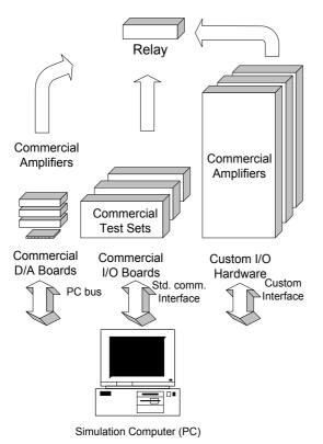
Fig. I. An advanced hardware configuration of an open-loop simulator
