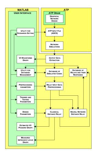
Fig. V. A new software for power system modelling and simulation as well as protective relay design and evaluation
