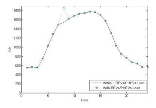
Fig. 3. Impacts of faster charging BEV/PHEVs on load demand.
