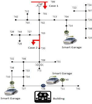
Fig. 5. Diagram of test feeder with smart garages.
