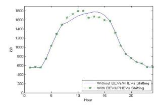
Fig. 4. Peak load shifting with BEVs/PHEVs for a typical summer daily load.
