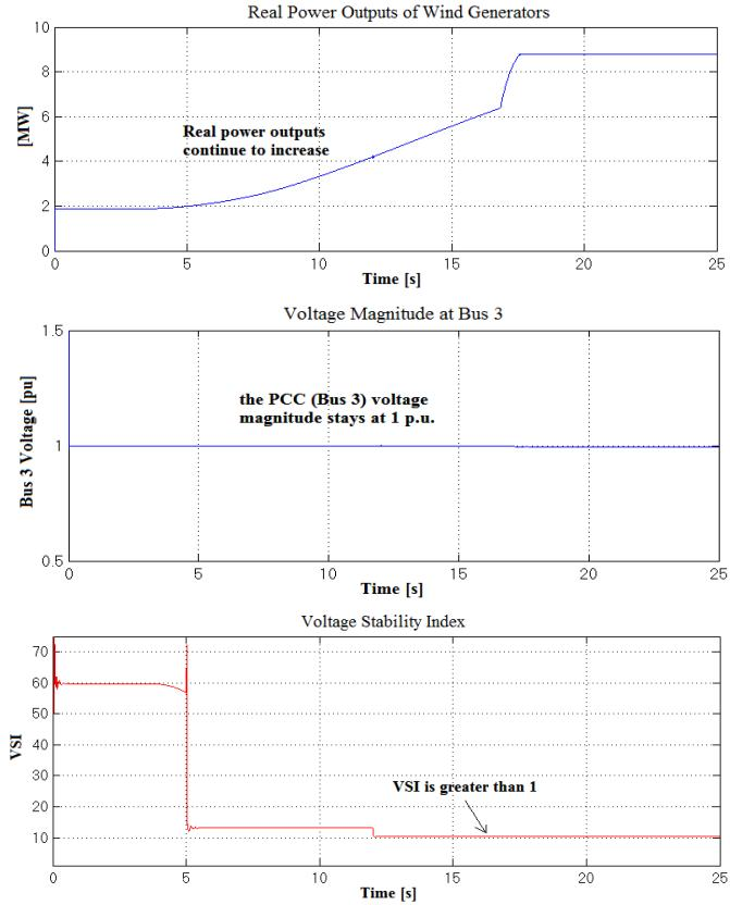
Fig. 8. Simulation results of DFIG-based wind farm with load and without additional reactive power compensation
