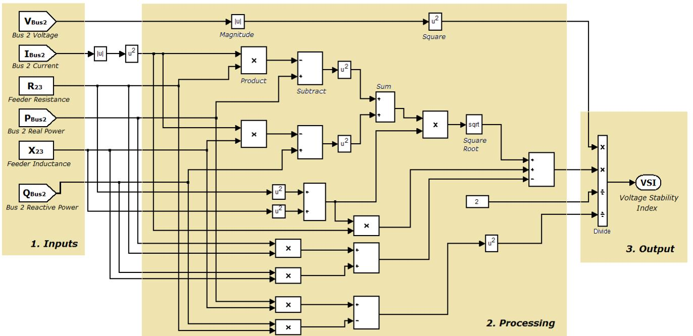
Fig. 4. Voltage Stability Index implemented in Matlab/Simulink
