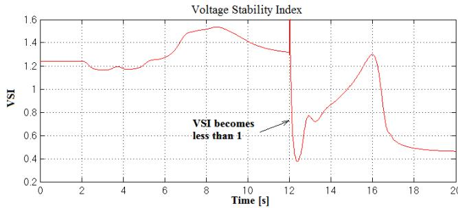
Fig. 5. Simulation results of SCIG-based wind farm with the AC undervoltage with protection disabled
