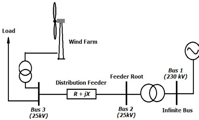
Fig. 2. Single line diagram of the test system with wind farm integration
