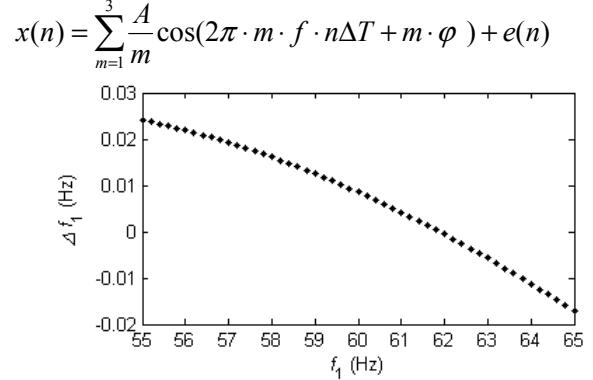
Fig. 3 Fundamental frequency error
