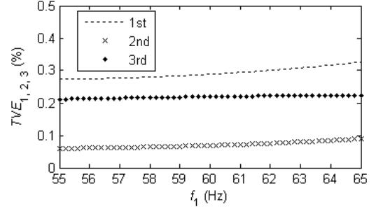
Fig. 4 Total vector error of harmonic components
