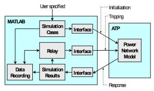
Figure 4. An Example of Integrated Simulation Tools for Protective Relaying by Using MATLAB and ATP
