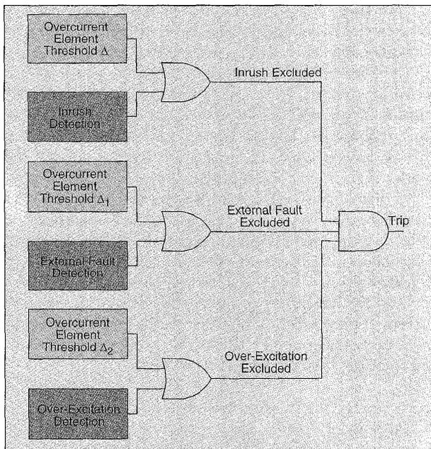
**Figure 4. Application of the overcurrent principle with multiple settings**
