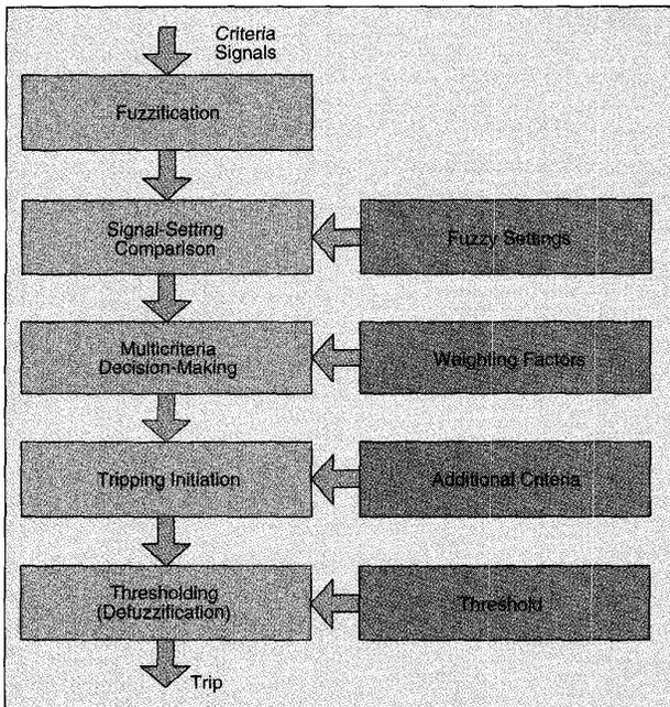
Figure 5. Fuzzy logic protective relay
