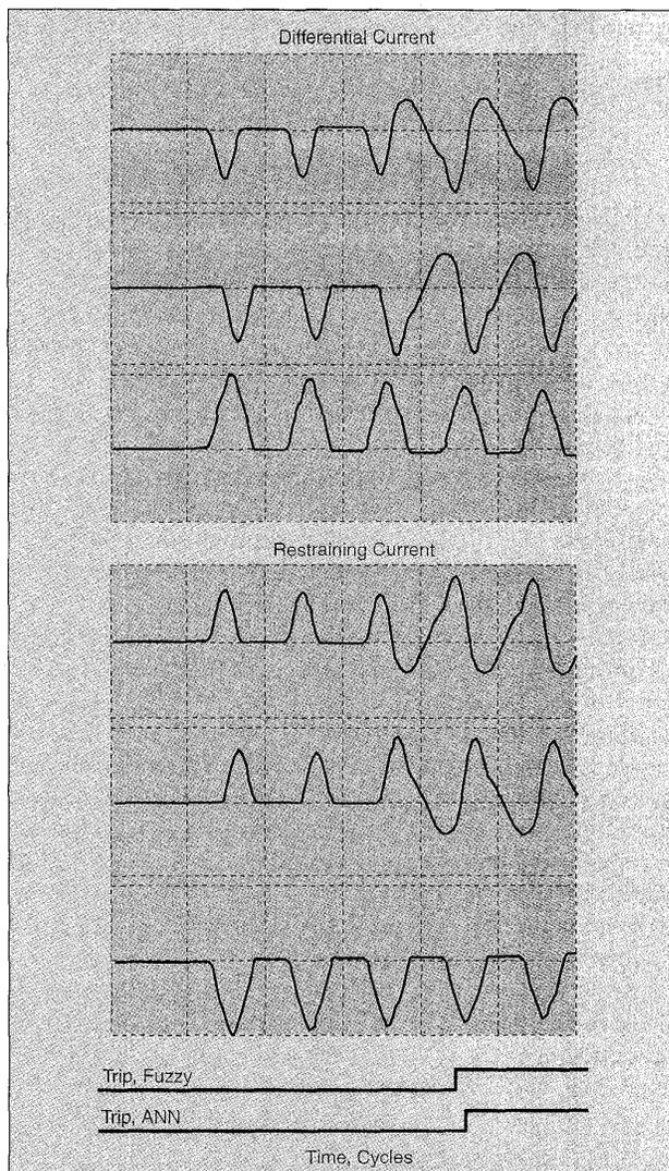
**Figure 7. Differential and restraining currents during an internal fault occurring in the course of transformer energization, and trip signals of the fuzzy-logic and ANN based transformer relays**
