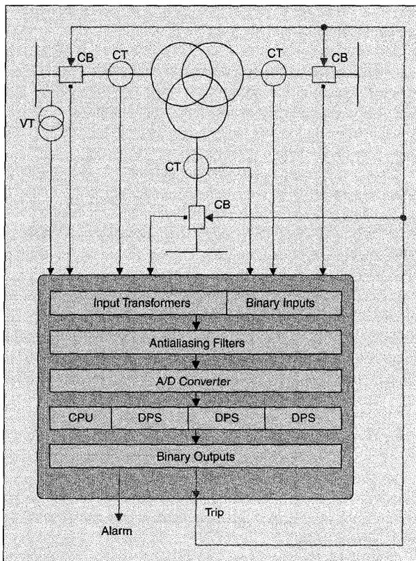
Figure 1. Hardware structure of a digital relay for power transformers
