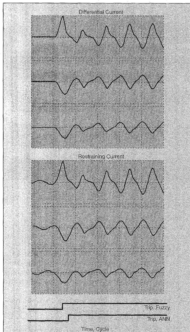
**Figure 8. Differential and restraining currents during an internal fault with deep saturation of the CTs, and trip signals of the fuzzy-logic and ANN based transformers relays**
