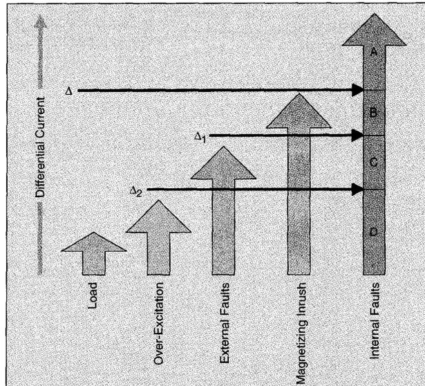
Figure 3. Multisetting overcurrent principle
