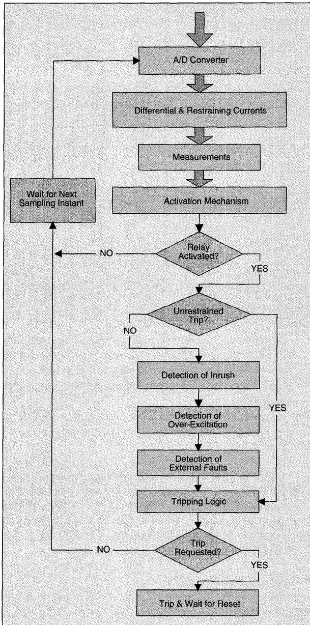
Figure 2. Logic for a digital differential relay for power transformers
