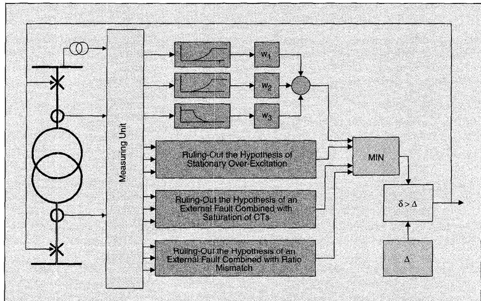
Figure 6. Fuzzy logic differential relay for power transformers
