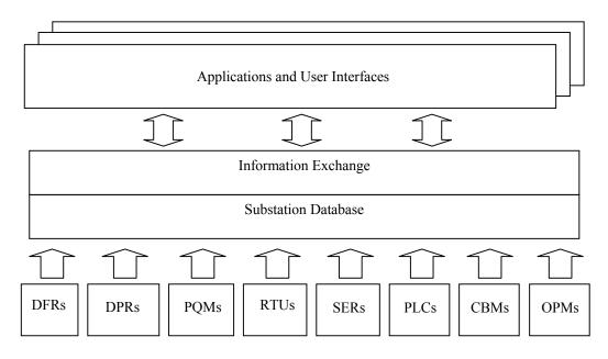
Figure 4. Data sources in a substation automation system
