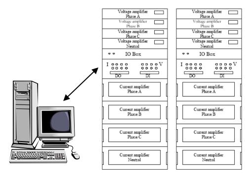
Figure 1. Two-terminal laboratory set-up
