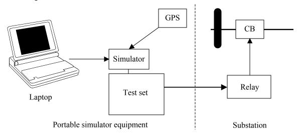
Figure 2. Portable simulator setup
