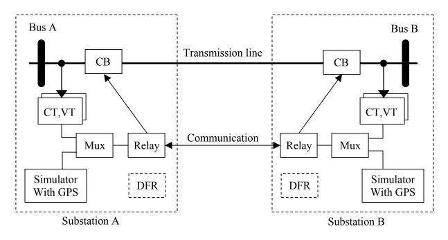
Figure 3. Digital simulator permanently installed in substations
