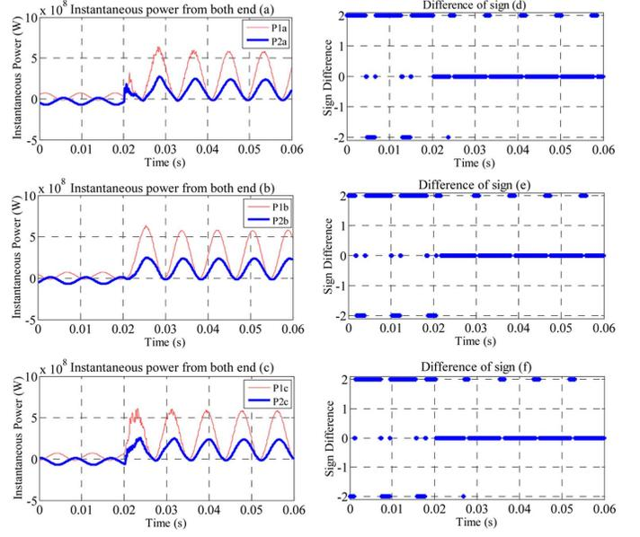
Fig. 6. (a)–(c)  $P_1(t)$  and  $P_2(t)$  with respect to time for the “abc” fault. (d)–(f)  $P_{sgn}(t)$  with respect to time for the “abc” fault.
