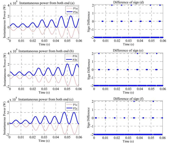
Fig. 7. (a)–(c)  $P_1(t)$  and  $P_2(t)$  with respect to time for the load level change. (d)–(f)  $P_{sgn}(t)$  with respect to time for the load level change.
