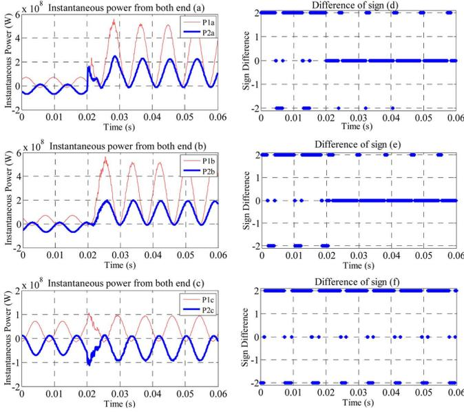
Fig. 4. (a)–(c)  $P_1(t)$  and  $P_2(t)$  with respect to time for the “abg” fault. (d)–(f)  $P_{sgn}(t)$  with respect to time for the “abg” fault.
