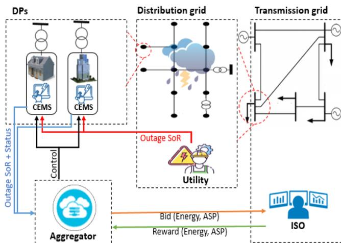
FIGURE 2. Coordination among aggregator, DPs, utility, and ISO.
