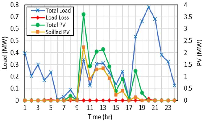
FIGURE 9. The DP resource management algorithm’s performance in load loss and PV power spillage prevention for the 5-day case study.
