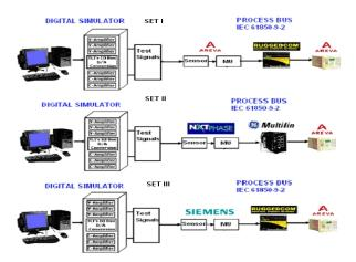
Fig. 12 Substation process bus test system.
