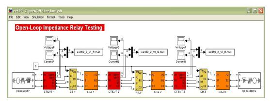
Fig. 14 Open-loop relay testing model.
