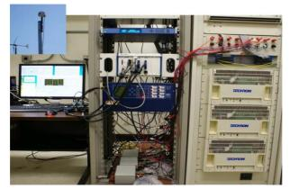
Fig. 11 Synchrophasor test system.
