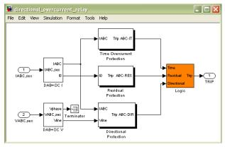
Fig. 4 Structure of directional overcurrent relay model.
