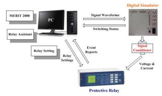
Fig. 9 Block diagram of relay test system.
