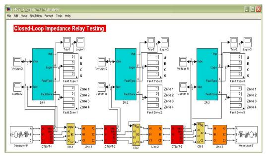
Fig. 13 Closed-loop impedance relay testing model.
