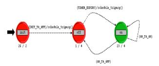
Fig. 7 Example of a protection IED process model.
