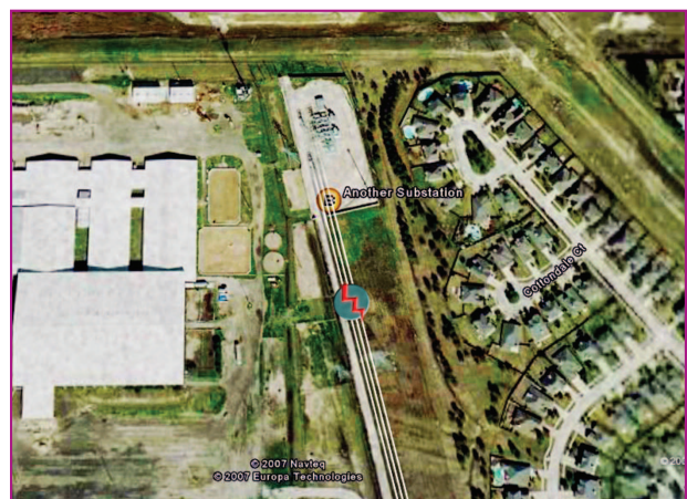
figure 17. Integration with a third-party visualization: displaying the calculated fault location on a satellite map.
