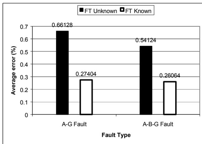
Fig. 4. The average error (%) of fault location.
