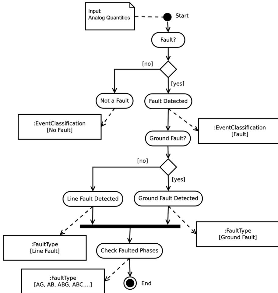
Figure 3. Fault detection and classification activity diagram.
