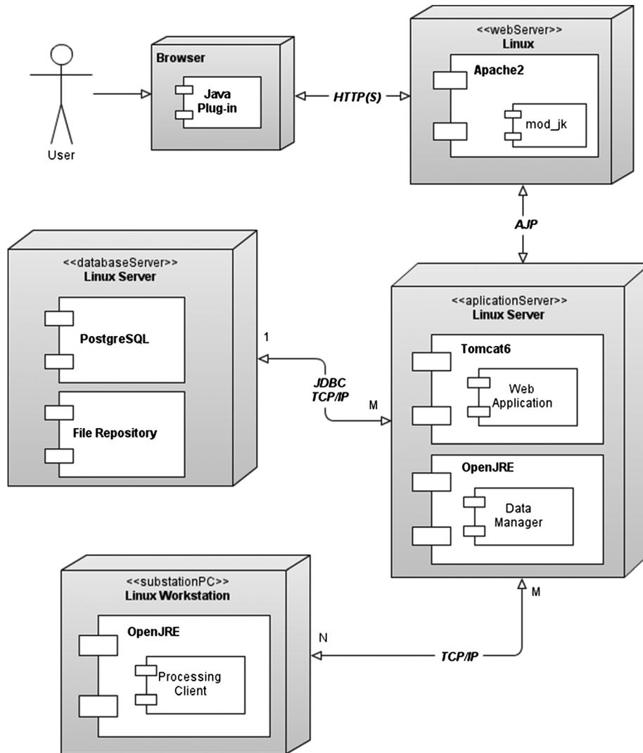
Figure 12. Solution deployment using open source software tools.
