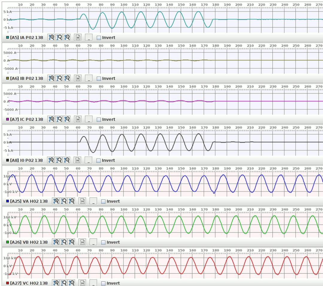
Figure 1. DFR event record triggered by an A-G fault on a transmission line.
