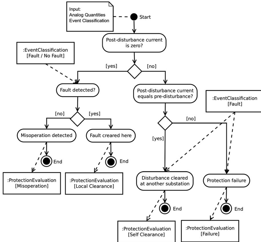
Figure 5. Protection evaluation activity diagram.
