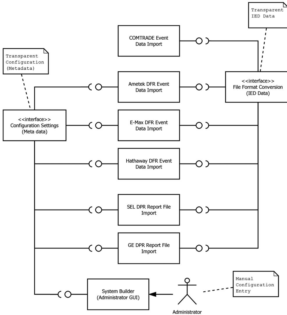
Figure 8. Implementation of the transparent data integration.
