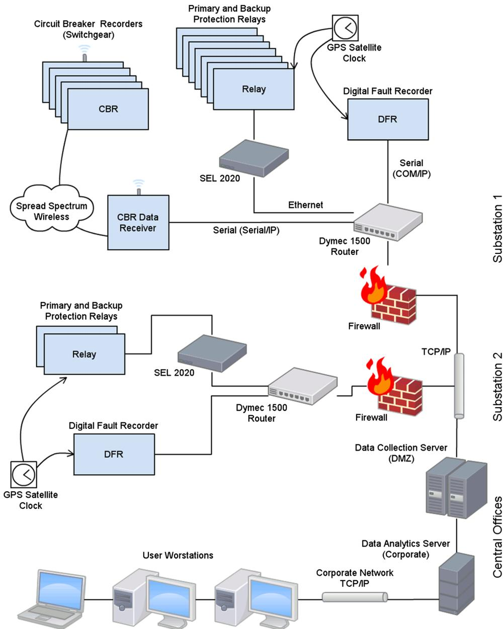
Figure 14. Field evaluation setup architecture and IED connection.
