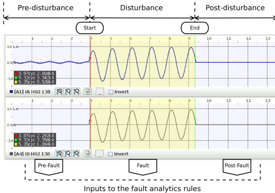
Figure 2. Identifying the disturbance start/end times, positioning the cursors.
