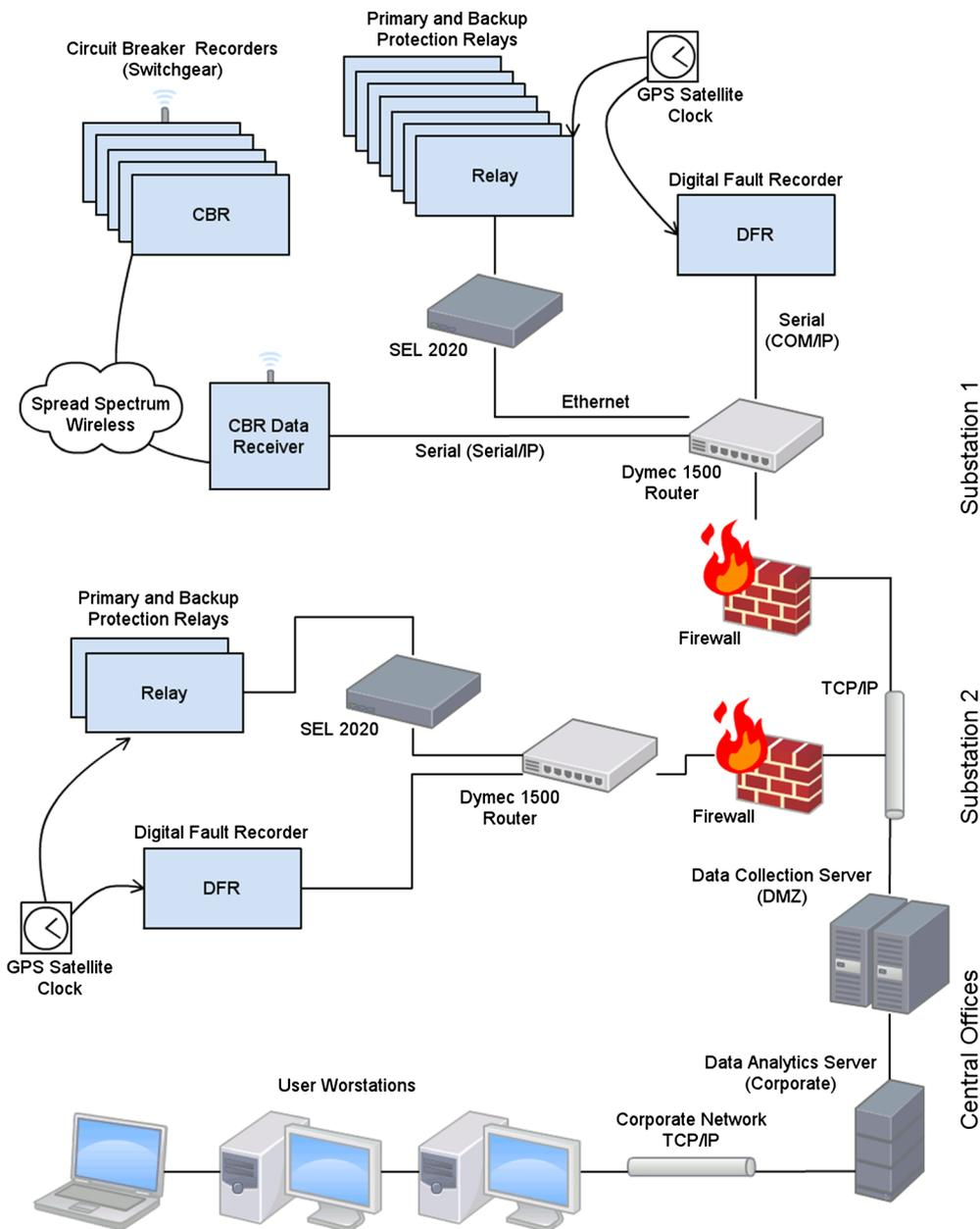
Figure 14. Field evaluation setup architecture and IED connection.
