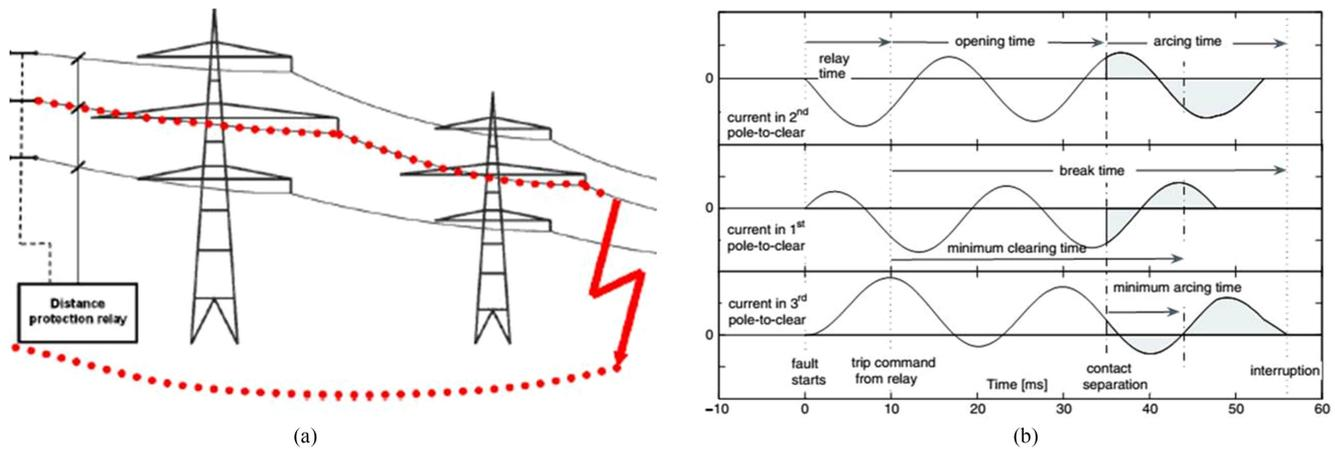
Fig. 1. (a) Faults in power systems. (b) CB three-phase current waveforms in the CB opening process to isolate the fault [37].
