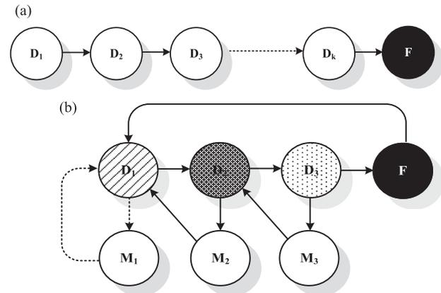
Fig. 4. (a) Classic state diagram for a deteriorating component over time. (b) Three-state deterioration/recovery state diagram with maintenance effects [32].
