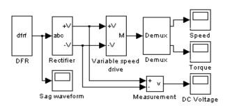
Fig.11. The testing diagram for the VSD
