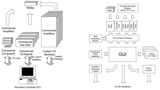
Fig. 9. The hardware architecture of the simulator Fig. 10. The software architecture of the simulator
