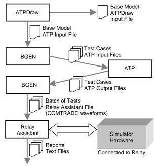
Fig. 4. Application testing setup
