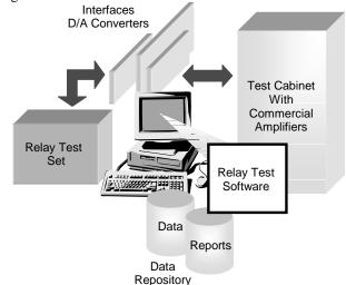
Fig. 2. The architecture of a PC-based open-loop simulator
