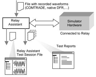
Fig. 3. Test setup for application testing using recorded waveforms
