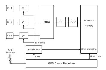
Fig. 1 Input channels data sampling and processing in a modern IED
