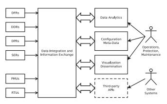
Fig. 2 Automated substation IED data analytics concept
