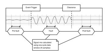
Fig. 4 Extracting phase current features with respect to the fault start and end
