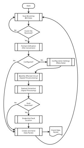
Fig. 5 Client implementation for the automated analysis of DPR files
