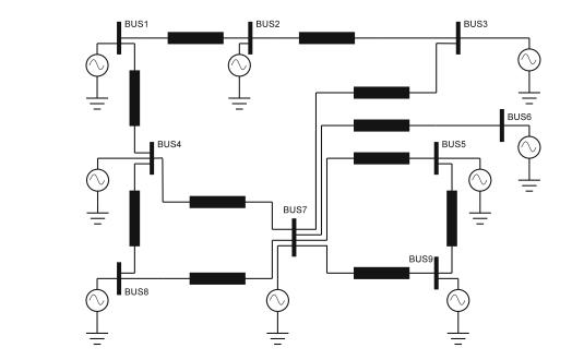
Fig. 8 An example 9-bus system model used for EMTP simulations
