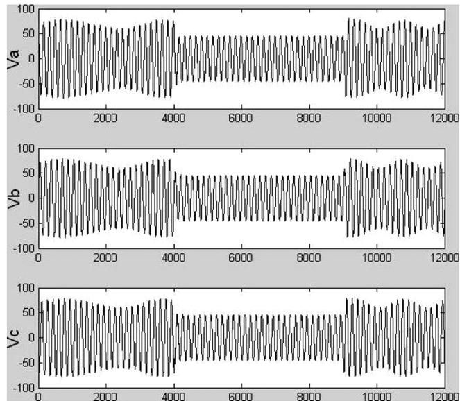
Fig. 12. Three phase voltage waveforms for a symmetrical fault during the power swing.
