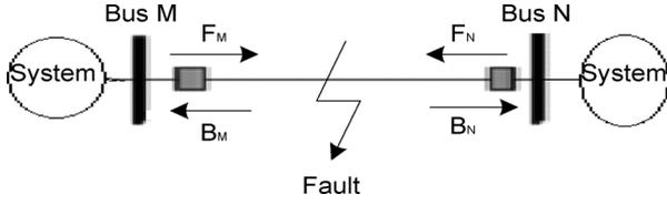
Fig. 2. Diagram for single phase transmission line.
