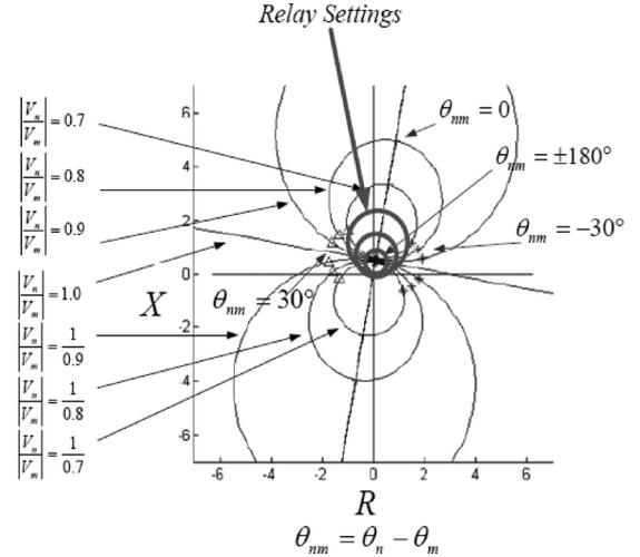
Fig. 1.  $Z_c$  trajectory in the  $R$ - $X$  phase.
