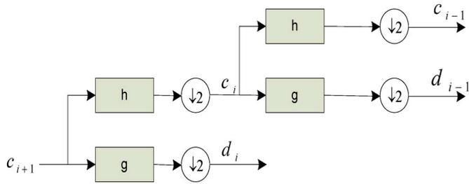
Fig. 3. Diagram of the MRA decomposition into two scales.
