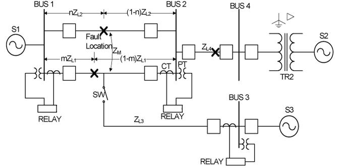
Fig. 9. One-line diagram of IEEE EMTP reference model.
