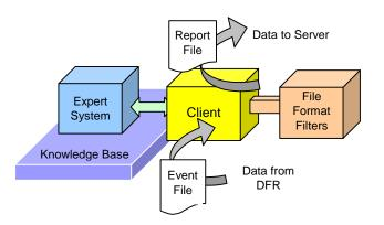
Figure 3: The architecture of Client
