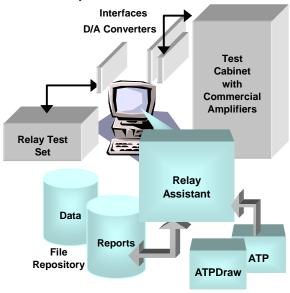
Fig. 4: The architecture of the simulator
