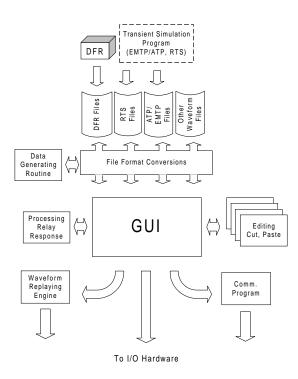
Fig. 2. The software architecture of the simulator
