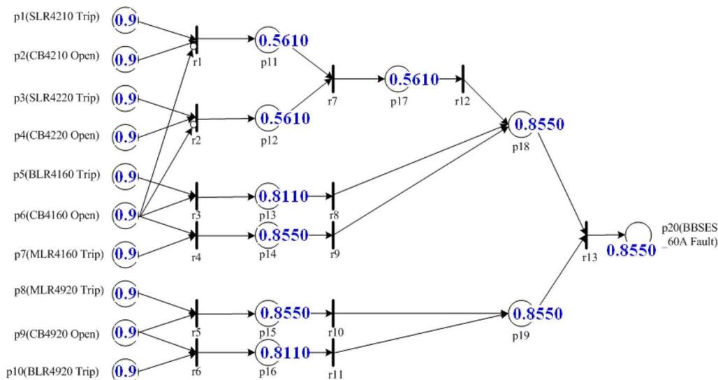
Fig. 12. FRPN model analysis procedure for line BBSES\_60A with assumed relay data.
