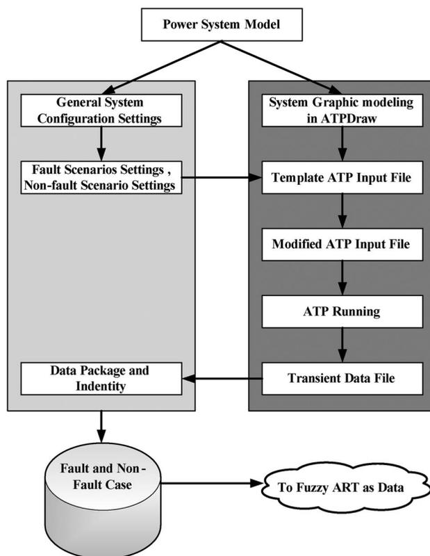
**Fig. 15.** Simulations for fault and nonfault scenarios.
