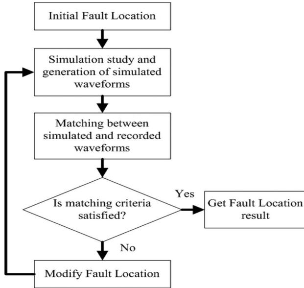
**Fig. 4.** Flowchart of system wide sparse measurement method.
