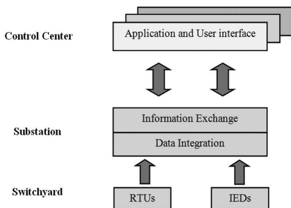
**Fig. 3. Functional diagram for substation data flow.**
