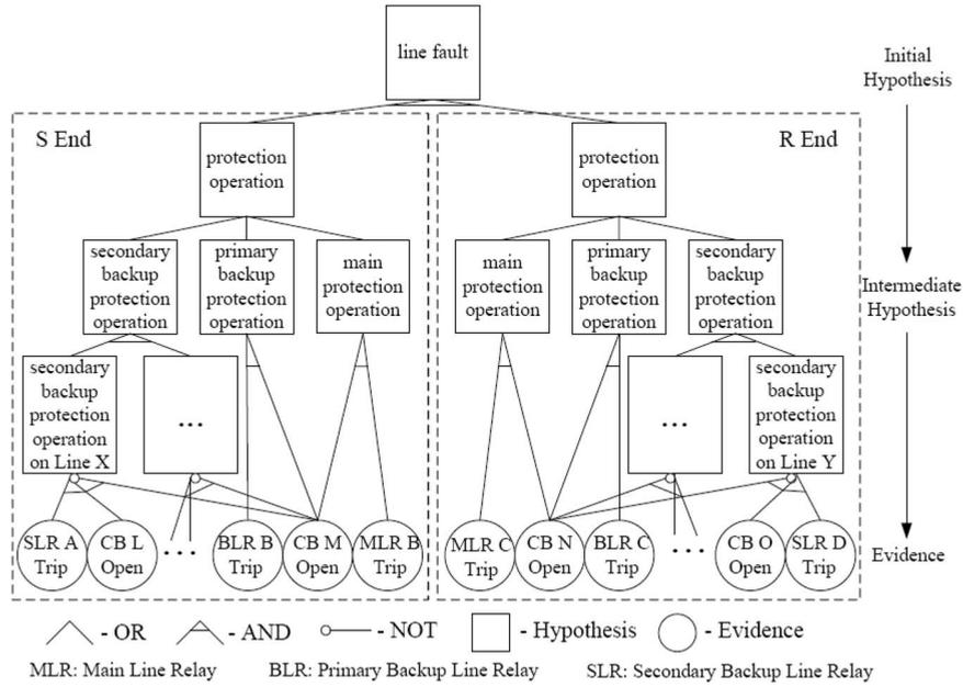
Fig. 7. Backward reasoning concept for structuring transmission line diagnosis models.
