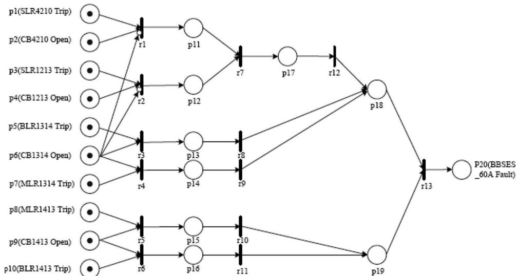
Fig. 8. A FRPN model for BBSES\_60A fault.
