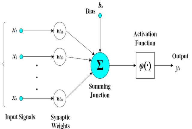
Fig. 13. Basic neuron model of a neural network.
