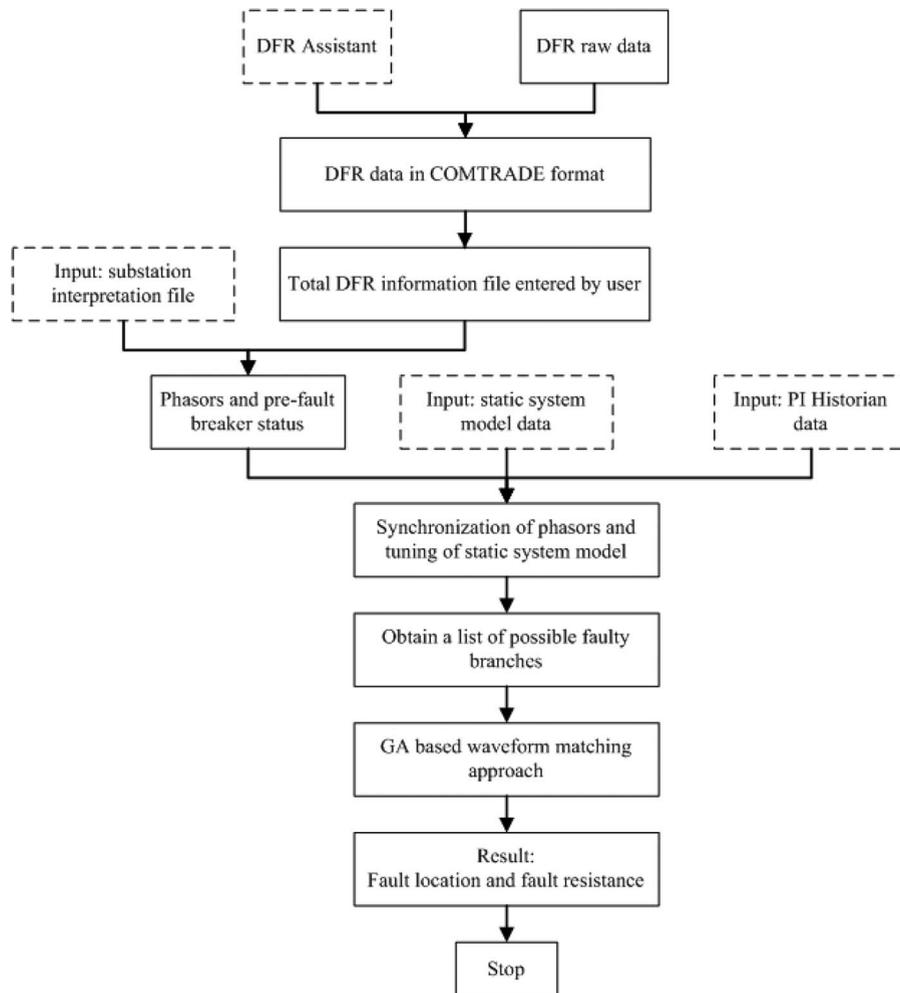
Fig. 5. Architecture of the fault location scheme.
