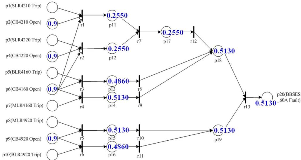
Fig. 11. FRPN model analysis procedure for line BBSES\_60A.
