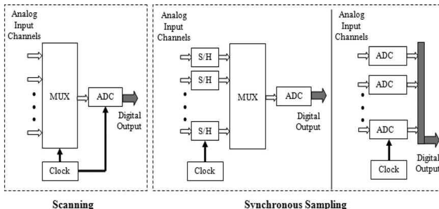
Fig. 1. Synchronous sampling versus scanning.
