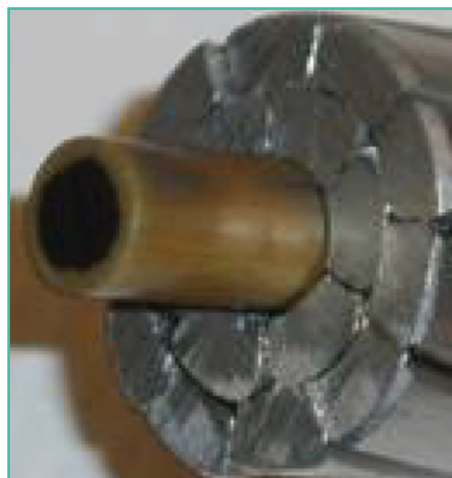
figure 3. Aluminum conductor composite core (ACCC) sample.
