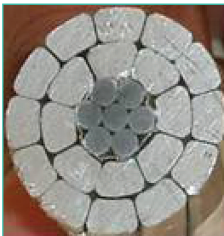
figure 2. Aluminum conductor composite reinforced (ACCR) sample evaluated for use as a high-temperature, low-sag overhead transmission conductor.
